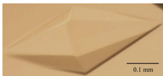
Figure 1 A crystal of recombinant Pz peptidase B obtained using 0.1 M bis-Tris–HCl pH 5.9, 2.3 M ammonium sulfate on earth. The crystal dimensions are about 0.5 \times 0.2 \times 0.1 mm. The scale bar is 0.1 mm in length.
